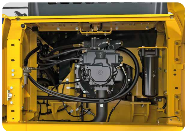
Pilot filter (Attachment piping specification)
