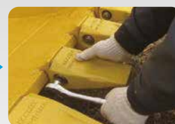
Set bushing, washer and bolt and tighten by a ratchet wrench.
