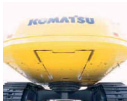
Strengthened revolving frame undercover
