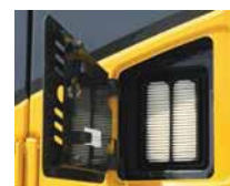
External air conditioner filter
