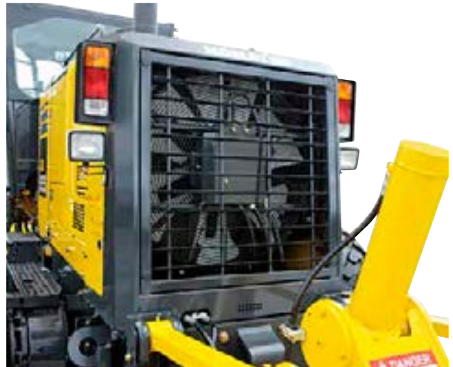
Hydraulic driven cooling fan
