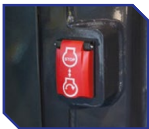
» Secondary engine shut down switch.
